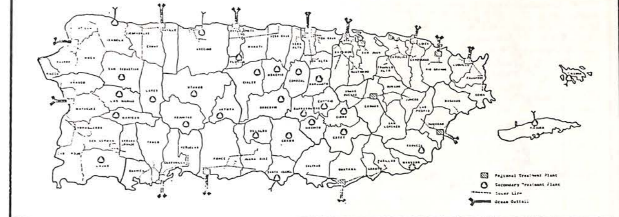
FIGURE 1-2: RECOMMENDED SEWFRAGE SYSTEM, ISLANDWIDE
